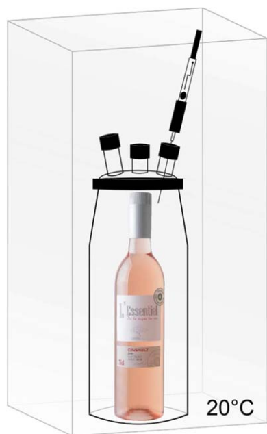
Figure 1. System used to evaluate permeation of aroma compounds through PET bottles. [Color figure can be viewed in the online issue, which is available at wileyonlinelibrary.com .]
